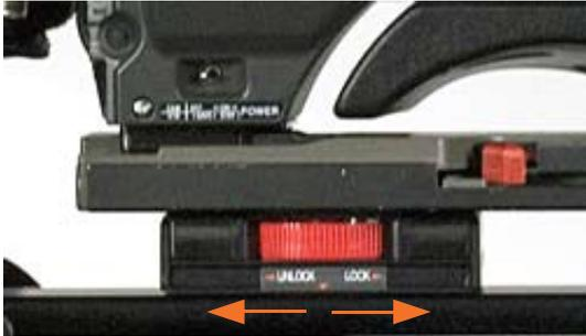
Turn knob to left to unlock and to the right to lock. Remove the cameras lens shade. Position camera lens within 1/2" from glass.
