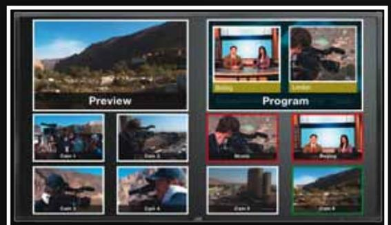
Includes internal high quality 10-input multiviewer and output routable to Preview or PGM-2 outputs and freely assignable source names.
